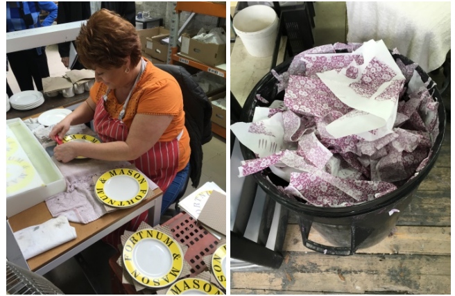
A Middleport Pottery worker demonstrates how to rub on the yellow transfers to a plate and then I found the trash with used and scrap purple transfers.
